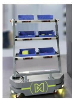
Each press of a flashing button, saves 12-20 seconds searching for a "pick". To kit a batch of parts, locate the flashing lights, pick the qty displayed, then press the button. Virtually no training required!
